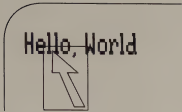
Figure 11-10. If a graphics cursor is accidentally overwritten (Figure 11-10a), a “hole” appears when the cursor is erased (Figure 11-10b).
